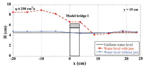
Figure 13. Measurements of water level with and without log jam at model bridge I.
