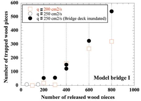
Figure 7. The number of wood pieces trapped by the model bridge I during water flow.
