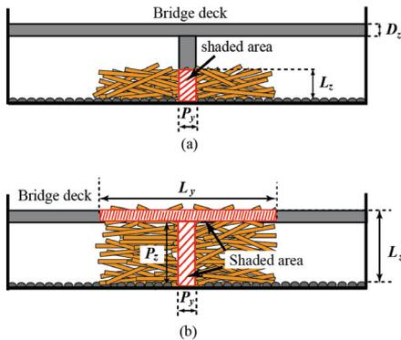
Figure 11. The definition of the ‘shaded area’ of an obstruction, such as the case of a jam formed by a pier (a) and that of a jam formed by bridge deck and pier (b).
