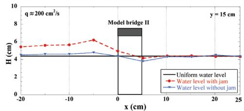
Figure 14. Measurements of water level with and without log jam at model bridge II.
