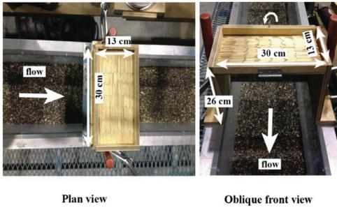
Figure 4. A basket used to drop wood pieces into the flume.
