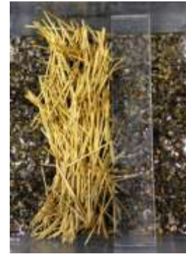
Figure 26. A top view of an accumulation at a bridge without piers.
