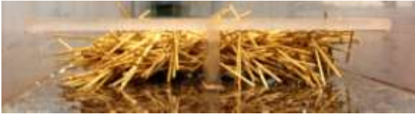
Figure 29. A front view of an accumulation at a bridge with a pier.
