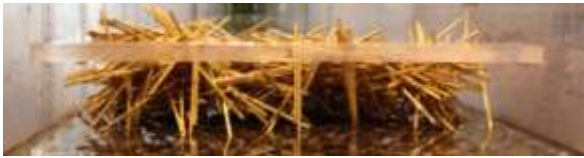
Figure 28. A front view of an accumulation at a bridge without piers.
