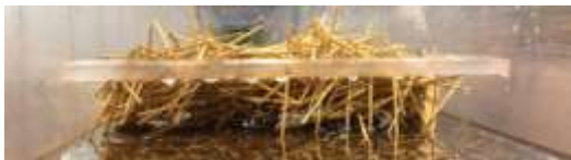
Figure 21. A front view of a typical woody debris accumulation formed at the model bridge after stopping the inflow.
