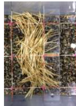
Figure 27. A top view of an accumulation at a bridge with a pier.
