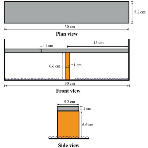
Figure 3. Model of Miyanoue Bridge (Model Bridge II).
