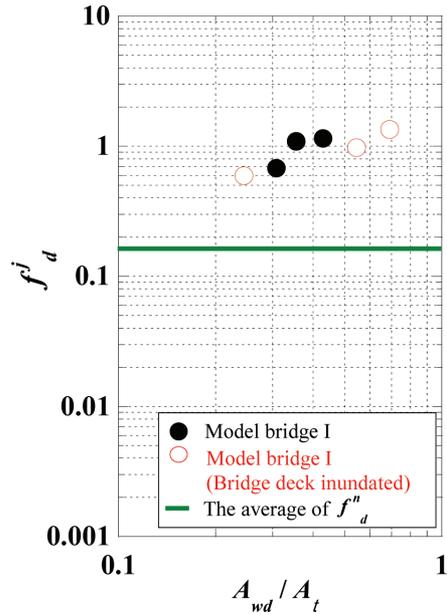
Figure 21. Relationship between the loss coefficient and the blockage ratio of jam.
