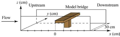
Figure 6. Definition sketch of the  $x$ ,  $y$  and  $z$  coordinates near the measurement point.
