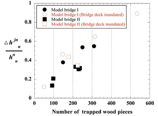
Figure 17. Relationship between the normalized backwater rise and the number of wood pieces trapped by a model bridge.
