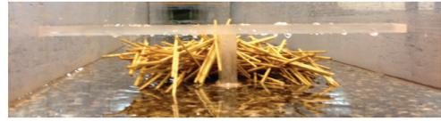
Figure 5. A front view of a typical log jam formed at model bridge I after stopping the inflow.
