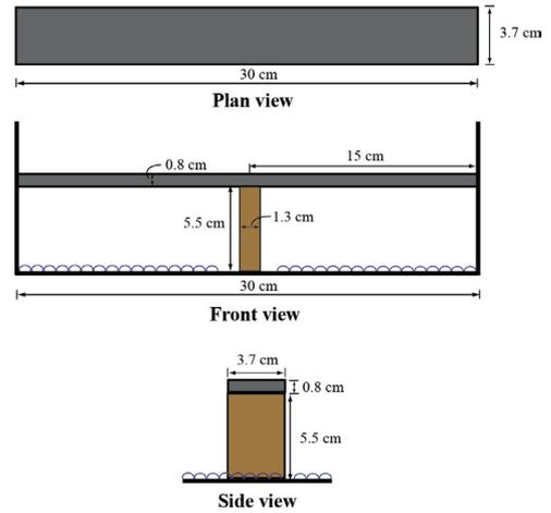
Figure 2. Model of Sokobarai Bridge (Model Bridge I).
