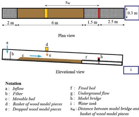
Figure 1. Experimental flume.
