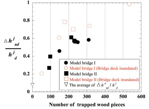
Figure 16. Relationship between the normalized backwater rise and the number of wood pieces trapped by a model bridge.
